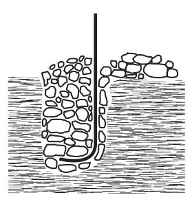
Requires over-backfill of trench **prior** to mechanical compaction.
